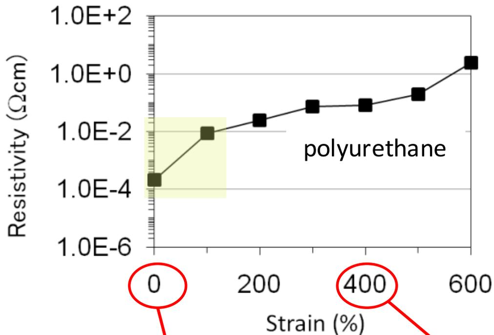
Good adhesion at interfaces provides ultra ductile wiring up to **600 %**
